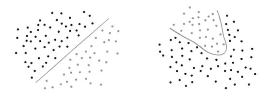
The figure on the left is linearly separable while the one on the right is not.
