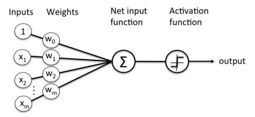
A perceptron follows the "feed-forward" model, meaning inputs are sent into the neuron, processed, and result in an output. In the diagram above, this means the network (one neuron) reads from left to right: inputs come in, output goes out.
