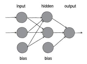
The above diagram is known as a *neural network*, a network of many neurons. Some are input neurons and receive the inputs, some are part of what's called a "hidden" layer (as they are connected to neither the inputs nor the outputs of the network directly), and then there are the output neurons, from which we read the results.
